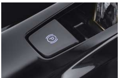
Electronic parking brake with auto-hold function
