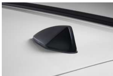
Shark-fin antenna with GLONASS, DAB and GSM
